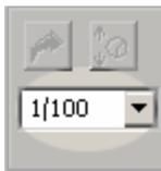
The log data display depth scale can be selected from this drop down list box at the extreme left of the panel.
