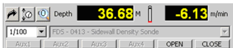
Fig. 1.2c Acquisition mode sonde powered on or replay mode with probe connected
