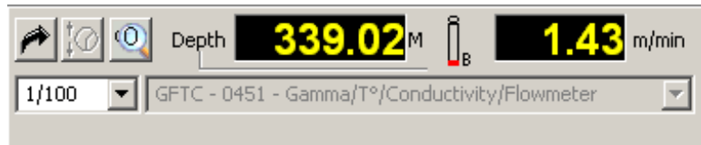
Fig. 1.2b Acquisition mode – probe powered off or replay mode with probe connected.
